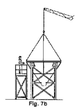
Steel gantry support and cone constructed at ground level and lifted to position. Constructed porizontal to be lifted by 2 cranes
