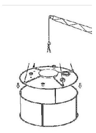
Silo top cone assembled first and lifted by crane. Lower rings bolted to top section in order and keep lifting and fitting a ring. 7 rings in total
