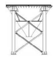
Full 7-ring silo top lifted to top of steel gantry & cone and fitted to position
